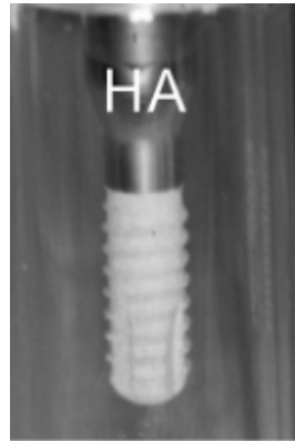
Figure 2. Titanium implant coated with hydroxyapatite [6].
